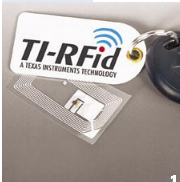
1. Tags inserted into key fobs can be used with vehicle mounted readers to unlock doors automatically as the driver approaches or to prevent the engine starting if the proper key is not present.
