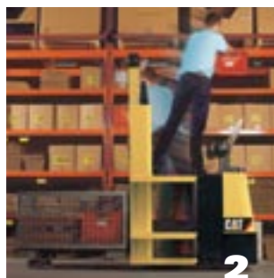
2. Line picking – in which individual pickers pick particular product lines for multiple orders
