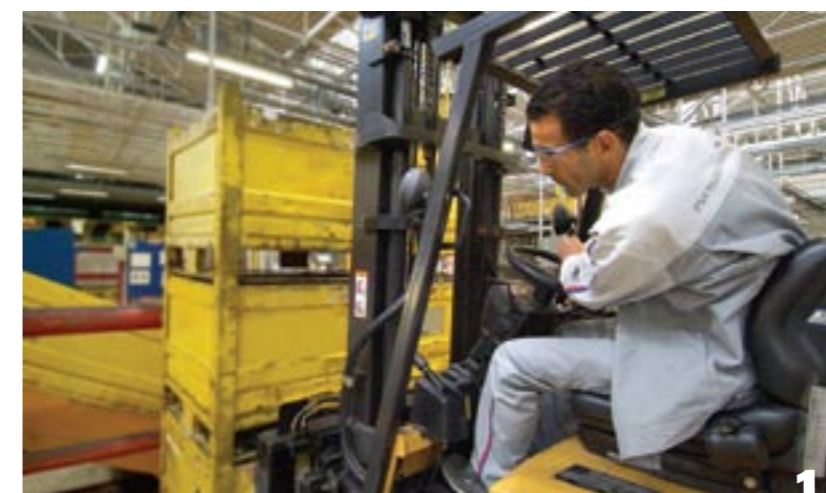
Main image: Forklifts are widely used within automotive manufacturing, where heavy production components are common. 1. An electric counterbalanced truck brings components to a car production line. (Image courtesy of PSA).
